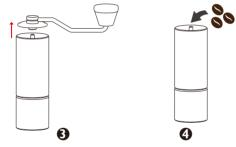
Fasten Body with the container. Then open the lid and pour coffee beans inside from the top of the grinder.
