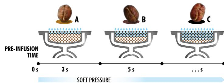
Pre-infusion is the first phase of espresso brewing. Its primary function is to saturate and prepare the coffee bed for optimal extraction. Pre-infusion also allows uniform delivery and aids in preventing channeling.
